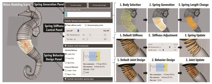
Figure 12. The *Ondulé* spring design tool interface (left) has four parts: Rhino modeling environment, a spring generation panel, a spring stiffness control panel, and a spring behavior design panel. The workflow for each design panel is shown on the right.
