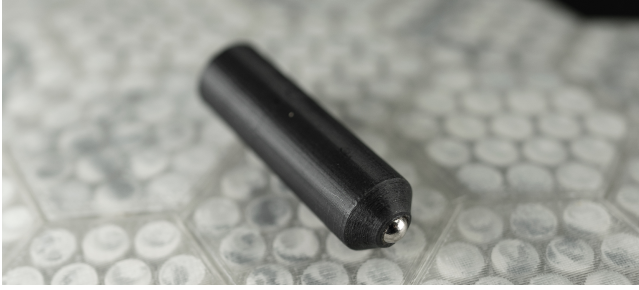
Figure 3: 3D printed erasing pen with a magnet. We use this magnetic pen to edit the printed displays showcased in this paper.
