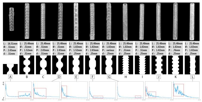
Figure 4. We conducted an informal exploration of corrugation variables that affect airflow, including: L: length, Ø: inner diameter, P: distance between corrugations, d: corrugation height. (Top row) actual 3D-printed tubes. (Middle row) corresponding diagrammatic views with parameters. (Bottom row) magnitude spectrums of signal generated through the representative corrugated tubes. The red rectangles in the plots highlight characteristically different energies across spectral signatures.
