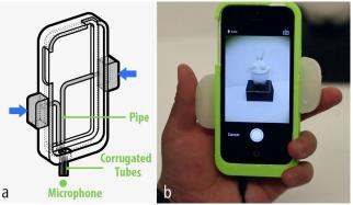
Figure 8. The smart case: (a) squeezing soft buttons generates air flows; (b) squeezing both buttons to take a photo.
