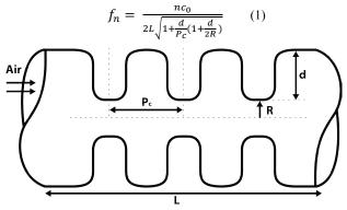
Figure 3. A corrugated tube diagram and equation.
