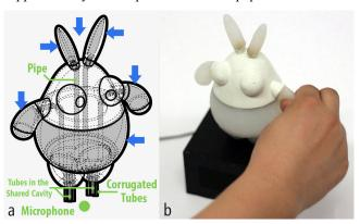
Figure 5. The interactive bunny: (a) interact with the bunny by squeezing soft parts (gray areas); (b) squeezing the bunny in real world. Blue arrows point to squeezable, interactive areas.
